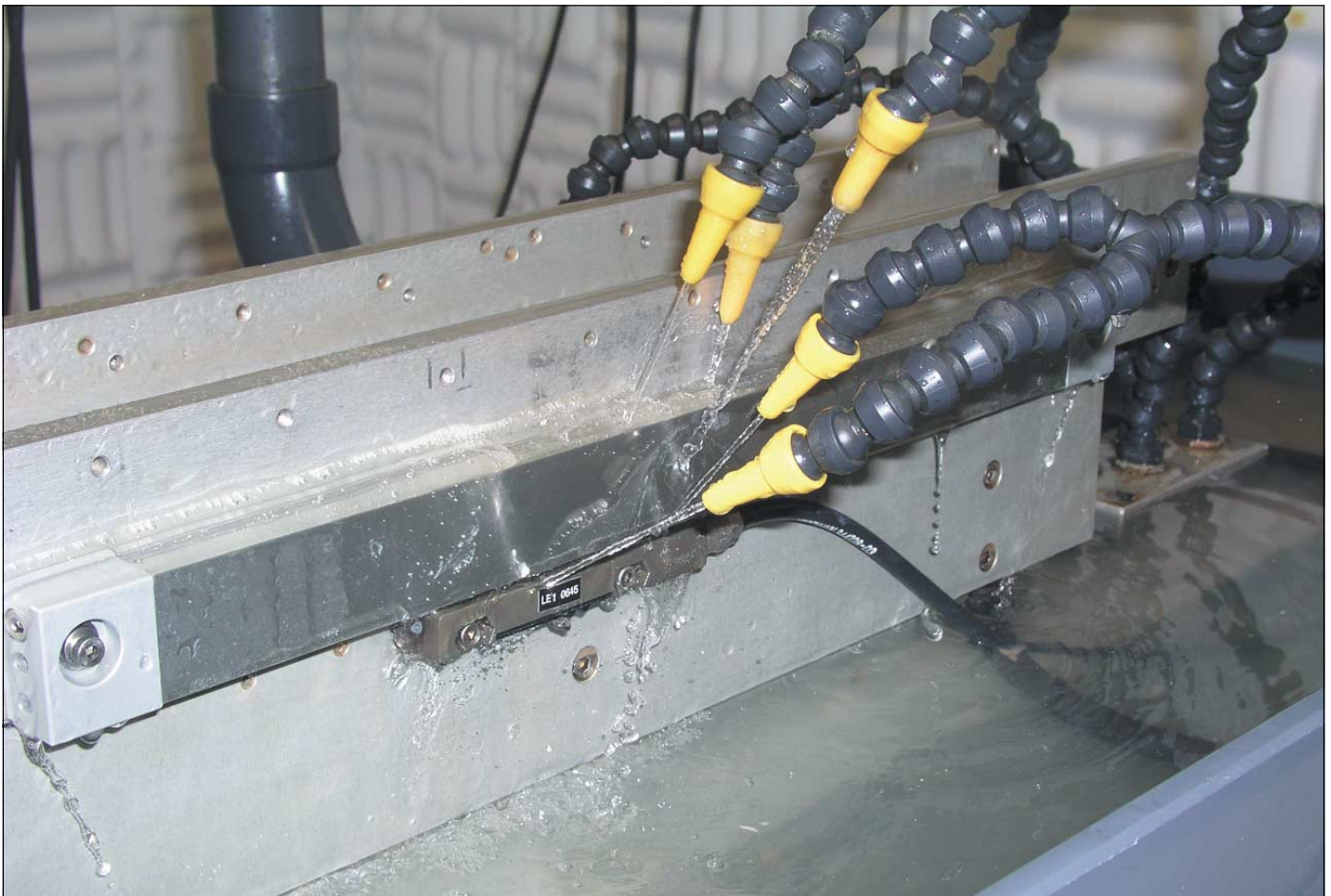
Splash test unit with slimline linear encoder
